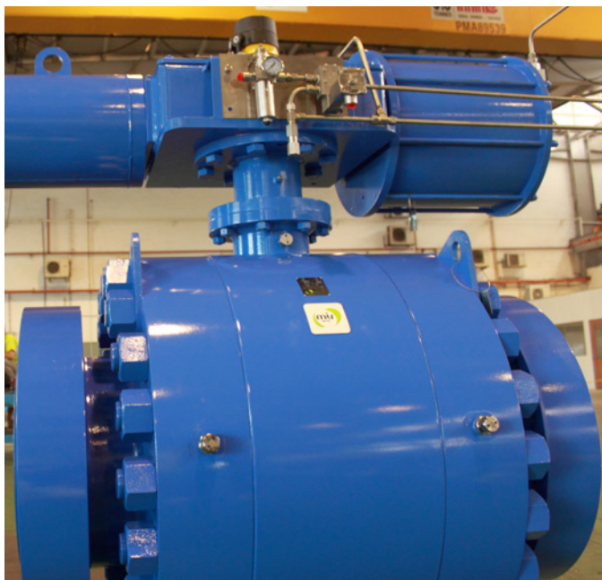
16" CL. 1500 full duplex, metal-seated +150 \mu TCC, PMI High-pressure gas testing as per API 598 Offshore Malaysia
